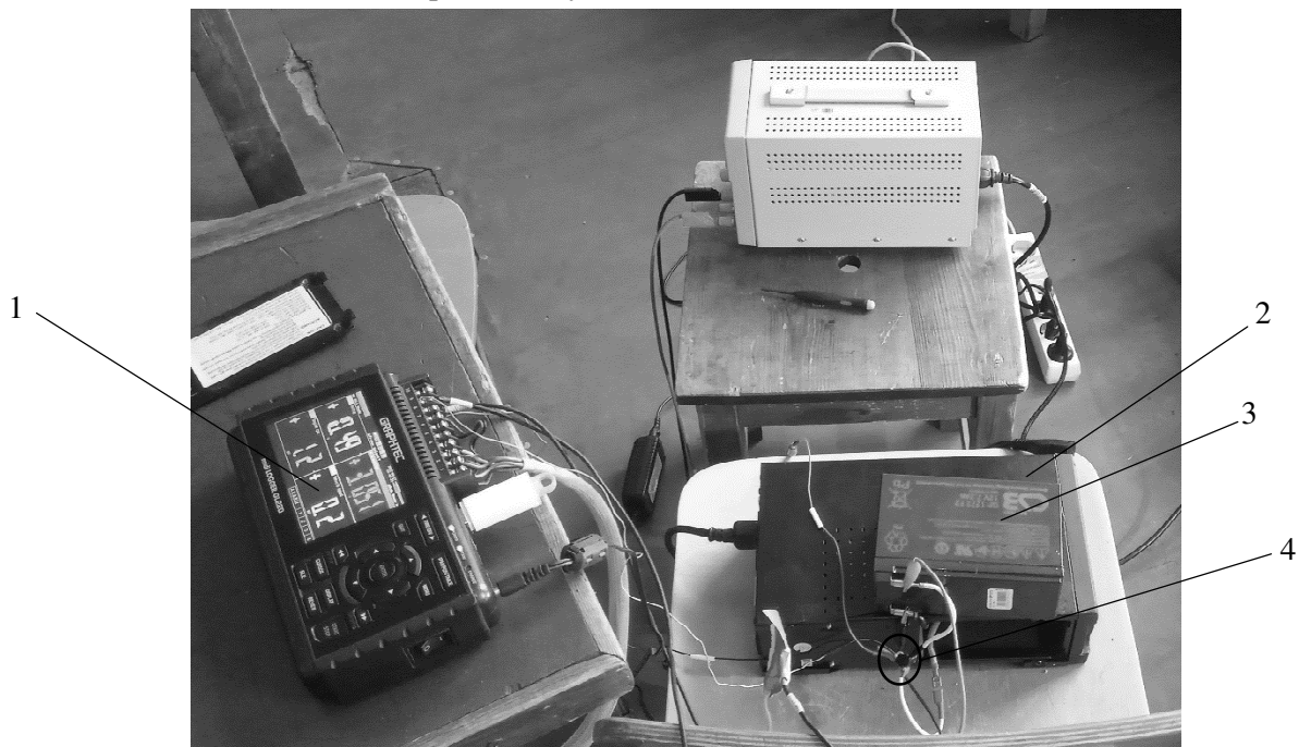
Fig. 4. Experiment setup: 1 – GL220 Logger; 2 – Test UPS device; 3 – UPS battery; 4 – ACS758 current sensor
